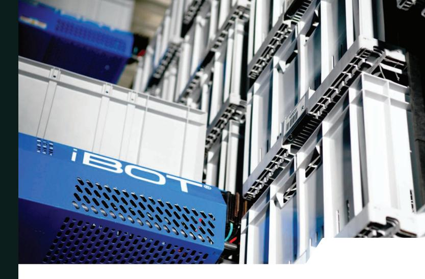
Perfect Pick's revolutionary "one-touch" design is based on the iBOT<sup>®</sup>, an autonomous robotic delivery vehicle with 100% access to all of the inventory in a single aisle. The energyefficient iBOTs store and retrieve totes and deliver them *directly* to the picking station at one or both ends of the aisle - without elevators, conveyors or transfers. Once the pick is completed, a new iBOT immediately appears for the next pick – no waiting or searching aisles for the next item.
