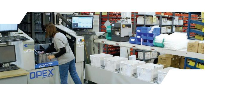
As individual items are picked, they are placed directly into shipping boxes or totes on the OPEX Workstation. The OPEX Workstation is closely integrated with Perfect Pick's hardware and software systems, reducing latencies and optimizing the overall system.
